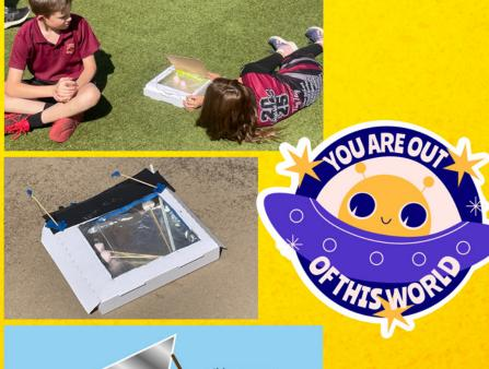
stick props open An example clear plastic wrap covers the "hole" in the pizza box aluminum foil -lines the bottom of the flap solar oven, similar to our inspiration. pizza box
